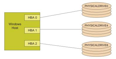
The next figure shows the same host after the cable attached to HBA0 has been removed and the host rebooted. Since Windows was not able to do a discovery on HBA0, it assigned **\PHYSICALDRIVE0** to the first device it discovered. In this case, that first device is connected to HBA1. Due to the shift, any software application accessing **\PHYSICALDRIVE0** will not find data previously written on the original **\PHYSICALDRIVE0**.
